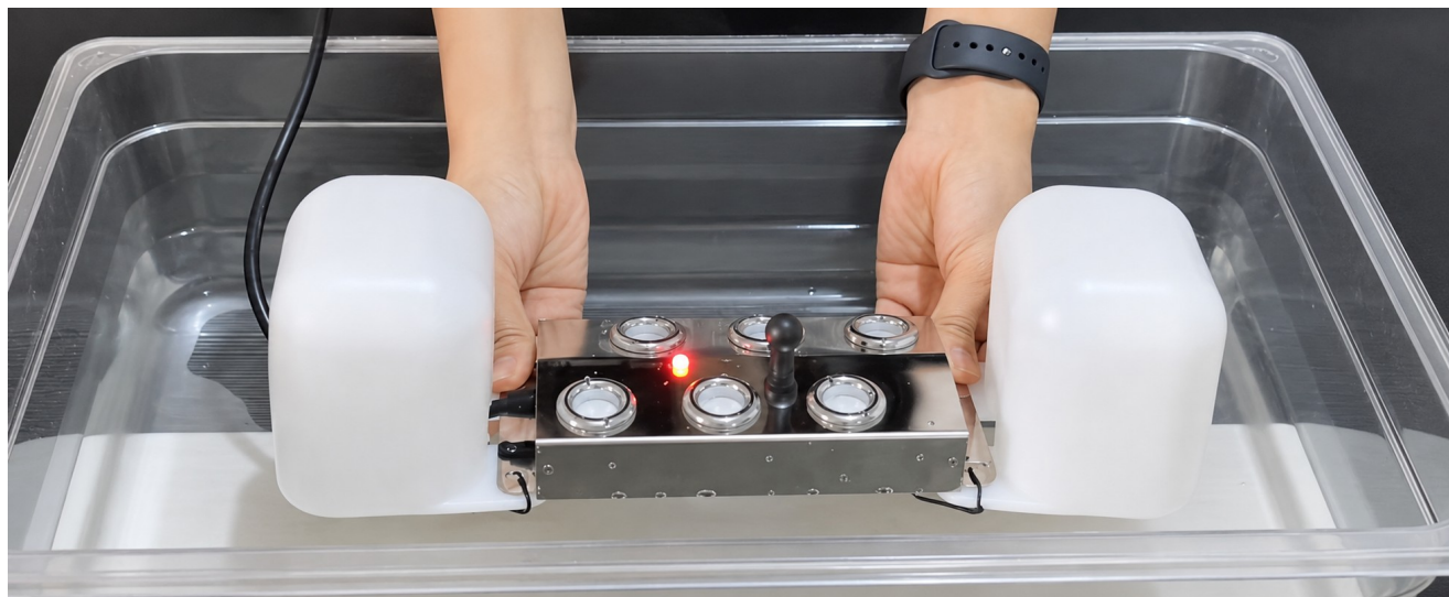
Figure 5-1. Installing the supplied float supports on a multi-head atomization module. Position the floats symmetrically and keep the module level.
