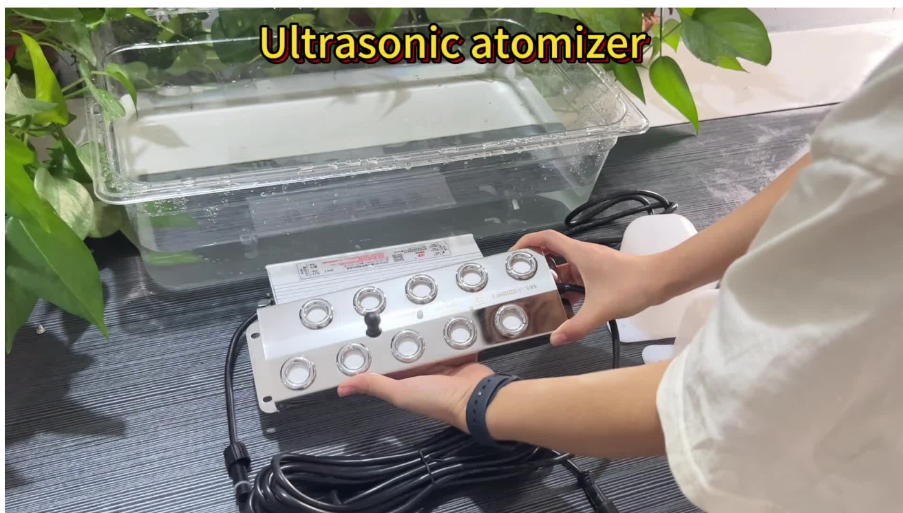
Typical MS multi-head module with matched waterproof power supply and accessories
