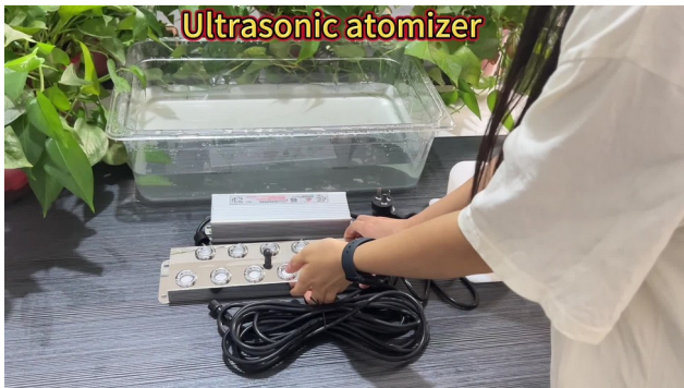
Figure A-8a. Actual MS-12 module and matched power supply
