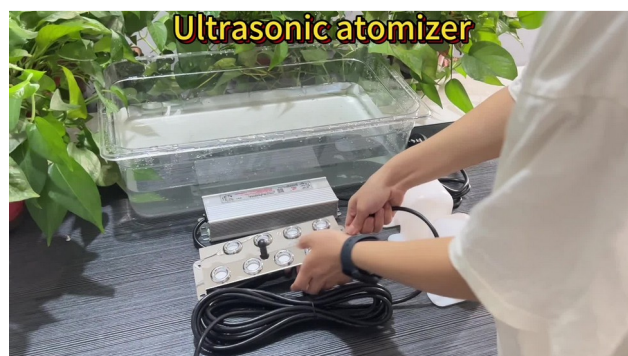
Figure A-6a. Actual MS-08 module and matched power supply
