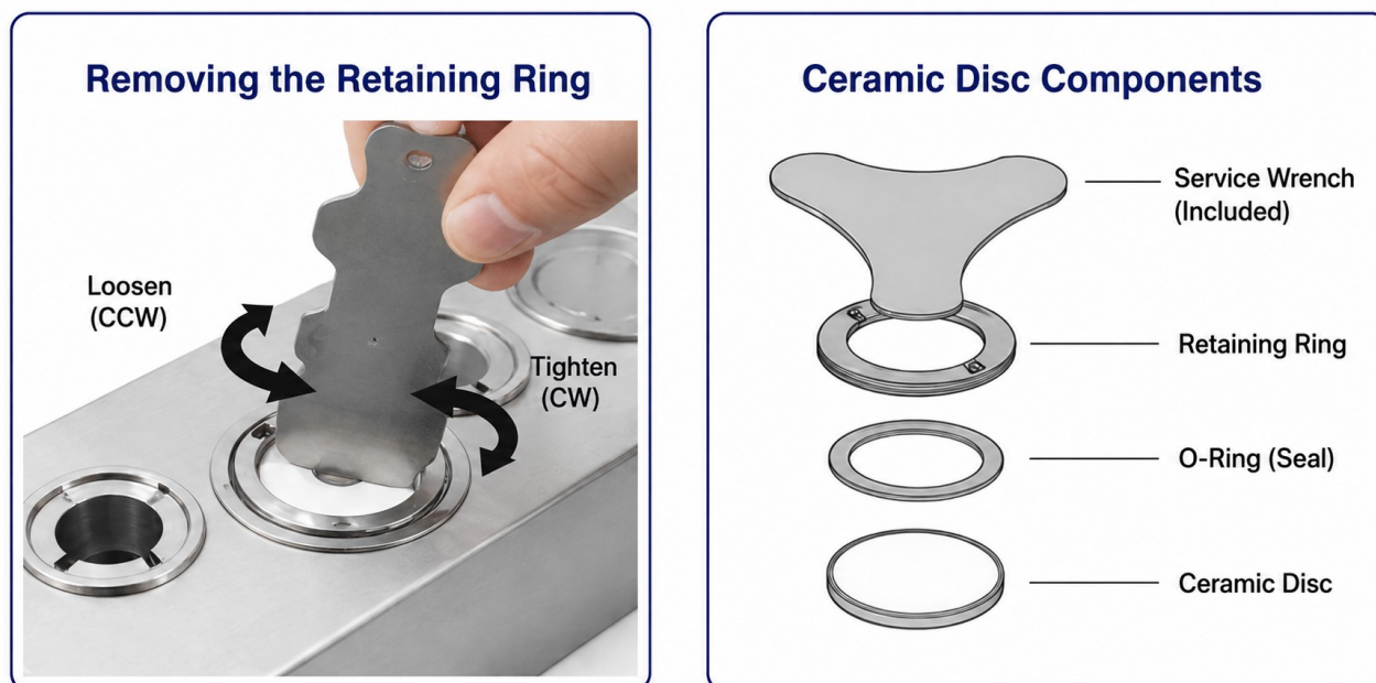
Figure 9-1. Retaining-ring direction and ceramic-disc component order.
