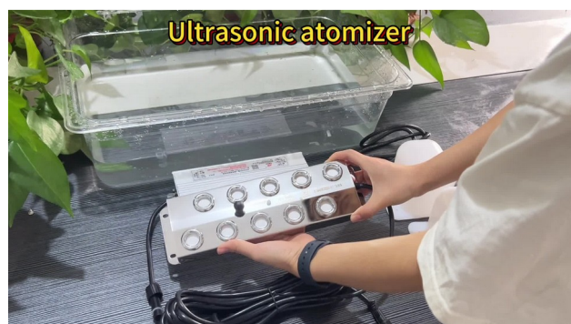
Figure A-7a. Actual MS-10 module and matched power supply
